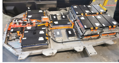
The real EV battery: students will study its structure and compartments in detail.
